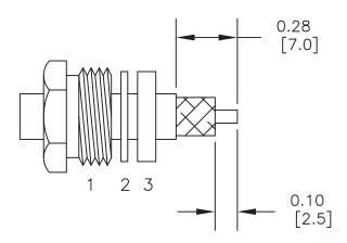
2. FORM BRAID OVER CLAMP NUT (4). SOLDER CONTACT TO CENTER CONDUCTOR. REMOVE EXCESS SOLDER. DO NOT OVER HEAT DIELECTRIC, INSERT CABLE ASSEMBLY INTO BODY & TIGHTEN.
