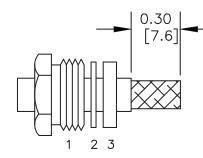
2. FORM BRAID OVER CLAMP NUT (4). TRIM BRAID BACK TO SHOULDER. CUT DIELECTRIC & CENTER CONDUCTOR TO DIMENSION SHOWN. DO NOT NICK CENTER CONDUCTOR. SOLDER CONTACT TO CENTER CONDUCTOR. REMOVE EXCESS SOLDER. DO NOT OVER HEAT DIELECTRIC. INSERT CABLE ASSEMBLY INTO BODY & TIGHTEN.
