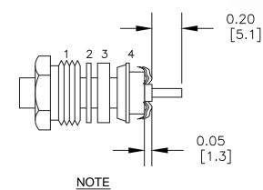
INSERT PTFE BEFORE CONTACT. WITH LARGE OPEN END SLIDING OVER CENTER CONDUCTOR & DIELECTRIC.
