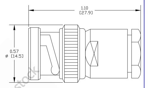
2. STRIP CABLE TO DIMENSION SHOWN. SLIDE SMALL WASHER (5) REAR INSULATOR (6) OVER DIELECTRICS. SOLDER CONTACTS (7) TO CENTER CONDUCTOR THROUGH HOLE IN CONTACT. CLEAN EXCESS SOLDER. SLIDE FRONT INSULATOR (8) OVER CONTACTS. SLIDE ASSEMBLY FORWARD INTO BODY & TIGHTEN.
