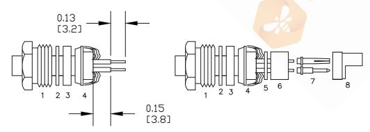
\* WHEN SOLDERING CONTACTS MAKE SURE SAME SEX IS ON BOTH ENDS OF WIRE IDENTIFIED BY THE BARE COPPER WIRE.
