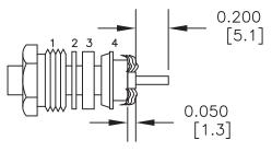
NOTE: INSERT PTFE BEFORE CONTACT. WITH LARGE OPEN END SLIDING OVER CENTER CONDUCTOR & DIELECTRIC.
