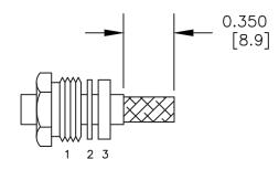
2. FORM BRAID OVER CLAMP NUT (4). TRIM BRAID BACK TO SHOULDER. CUT DIELECTRIC & CENTER CONDUCTOR TO DIMENSION SHOWN. DO NOT NICK CENTER CONDUCTOR. SOLDER CONTACT TO CENTER CONDUCTOR. REMOVE EXCESS SOLDER. DO NOT OVER HEAT DIELECTRIC. INSERT CABLE ASSEMBLY INTO BODY & TIGHTEN.
