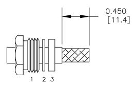
2. FORM BRAID OVER CLAMP NUT (4). TRIM BRAID BACK TO SHOULDER. CUT DIELECTRIC & CENTER CONDUCTOR TO DIMENSION SHOWN. DO NOT NICK CENTER CONDUCTOR. SOLDER CONTACT TO CENTER CONDUCTOR, REMOVE EXCESS SOLDER. DO NOT OVER HEAT DIELECTRIC. INSERT CABLE ASSEMBLY INTO BODY & TIGHTEN.
