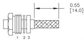
2. FORM BRAID OVER CLAMP NUT (4). TRIM BRAID BACK TO SHOULDER. CUT DIELECTRIC & CENTER CONDUCTOR TO DIMENSION SHOWN. DO NOT NICK CENTER CONDUCTOR. SOLDER CONTACT TO CENTER CONDUCTOR. REMOVE EXCESS SOLDER. DO NOT OVER HEAT DIELECTRIC. INSERT CABLE ASSEMBLY INTO BODY & TIGHTEN.
