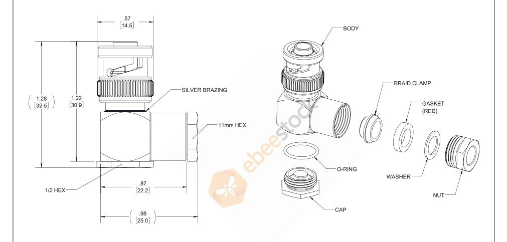
UNLESS OTHERWISE SPECIFIED LEADING DIMENSIONS ARE INCHES DIMENSIONS IN [] ARE MILLIMETERS
