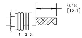
2. FORM BRAID OVER CLAMP NUT (4). TRIM BRAID BACK TO SHOULDER. CUT DIELECTRIC & CENTER CONDUCTOR TO DIMENSION SHOWN. DO NOT NICK CENTER CONDUCTOR, SOLDER CONTACT TO CENTER CONDUCTOR. REMOVE EXCESS SOLDER. DO NOT OVER HEAT DIELECTRIC. INSERT CABLE ASSEMBLY INTO BODY & TIGHTEN.
