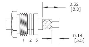
2. FORM BRAID OVER CLAMP NUT (4). SOLDER CONTACT TO CENTER CONDUCTOR. REMOVE EXCESS SOLDER. DO NOT OVER HEAT DIELECTRIC. INSERT CABLE ASSEMBLY INTO **BODY & TIGHTEN.**
