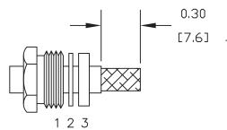
2. FORM BRAID OVER CLAMP NUT (4). TRIM BRAID BACK TO SHOULDER. CUT DIELECTRIC & CENTER CONDUCTOR TO DIMENSION SHOWN, DO NOT NICK CENTER CONDUCTOR.
