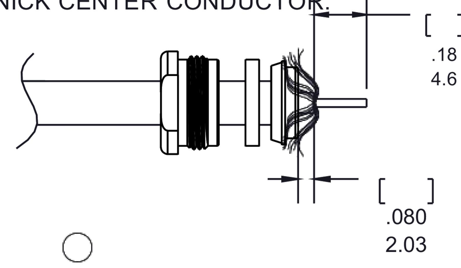
3. SOLDER CONTACT 4 TO CENTER CONDUCTOR. REMOVE EXCESS SOLDER. DO NOT OVER HEAT DIELECTRIC.INSERT CABLE ASSEMBLY INTO BODY 5 & TIGHTEN.
