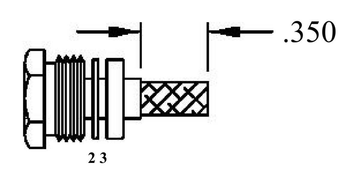
2. FORM BRAID OVER CMMP NUT (4). TRIM BRAID BACK TO SHOULDER. CUT DIELECTRIC & CENTER CONDUCTOR TO DIMENSION SHOWN. DO NOT NICK CENTER CONDUCTOR. SOLDER CONTACT TO CENTER CONDUCTOR. REMOVE EXCESS SOLDER. DO NOT OVER HEAT DIELECTRIC. INSERT CABLE ASSEMBLY INTO BODY & TIGHTEN.
