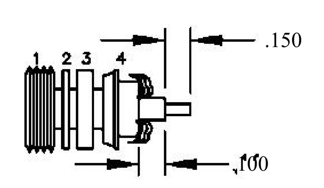
NOTE: INSERT PTFE BEFORE CONTACT. WITH OPEN END SLIDE OVER CENTER CONDUCTOR RESTING AGAINST DIELECTRIC.
