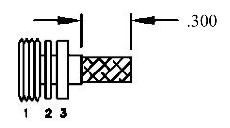
CLAMP NUT (4). TRIM BRAID BACK TO SHOULDER. CUT 2. FORM BRAID OVER DIELECTRIC & CENTER CONDUCTOR TO DIMENSION SHOWN. DO NOT NICK CENTER CONDUCTOR. SOLDER CONTACT TO CENTER CONDUCTOR. REMOVE EXCESS SOLDER. DO NOT OVER HEAT DIELECTRIC. INSERT CABLE ASSEMBLY INTO BODY & TIGHTEN.
