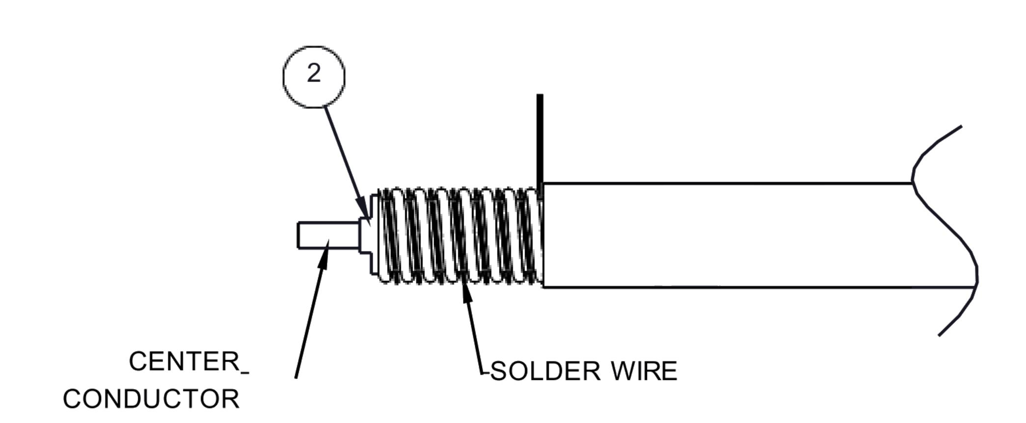
3. PUSH THE CONNECTOR BODY INTO THE CABLE, UNTIL IT STOPS. SOLDER THE CONNECTOR BODY WITH CABLE. SOLDER THE INNER CONDUCTOR. PRESS THE CAP (FINTO BODY AND COVER HEATSHRINK SLEEVE.
