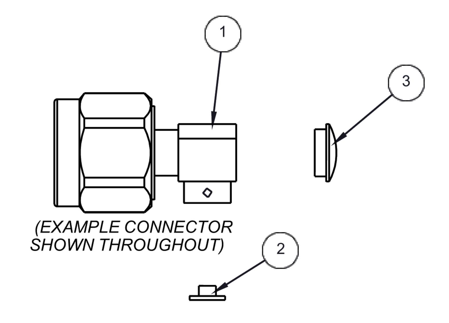
1. STRIP CABLE AS SHOWN, CHAMFER CENTER CONDUCTOR AND DEBURR CABLE.
