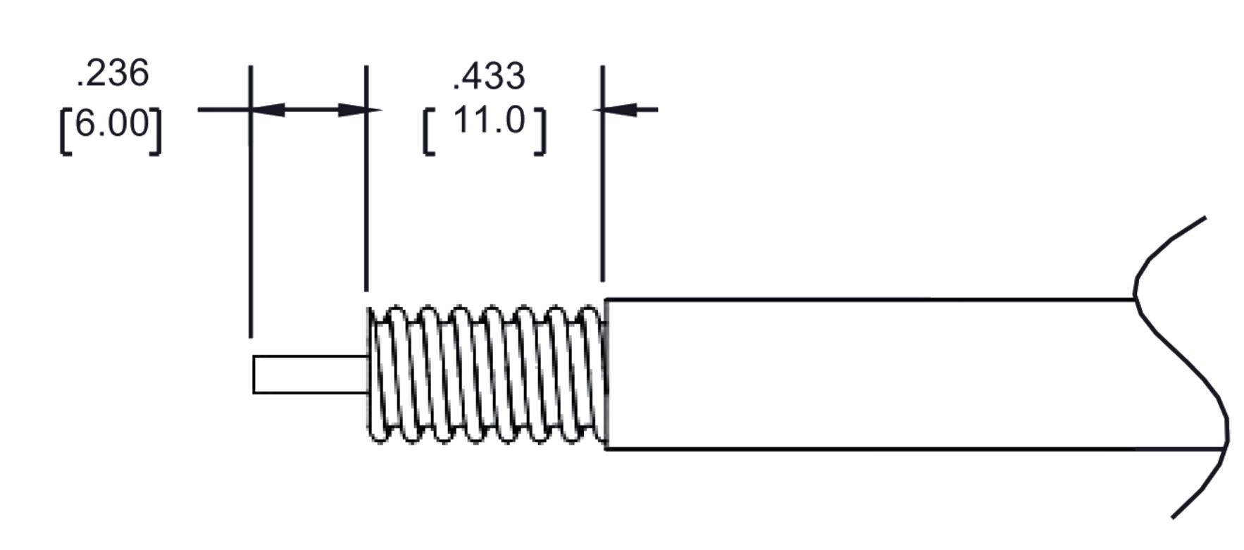
2. SLIDE INSULATOR FOVER CABLE CENTER CONDUCTOR AND WRAP THE CABLE BY SOLDER WIRE.
