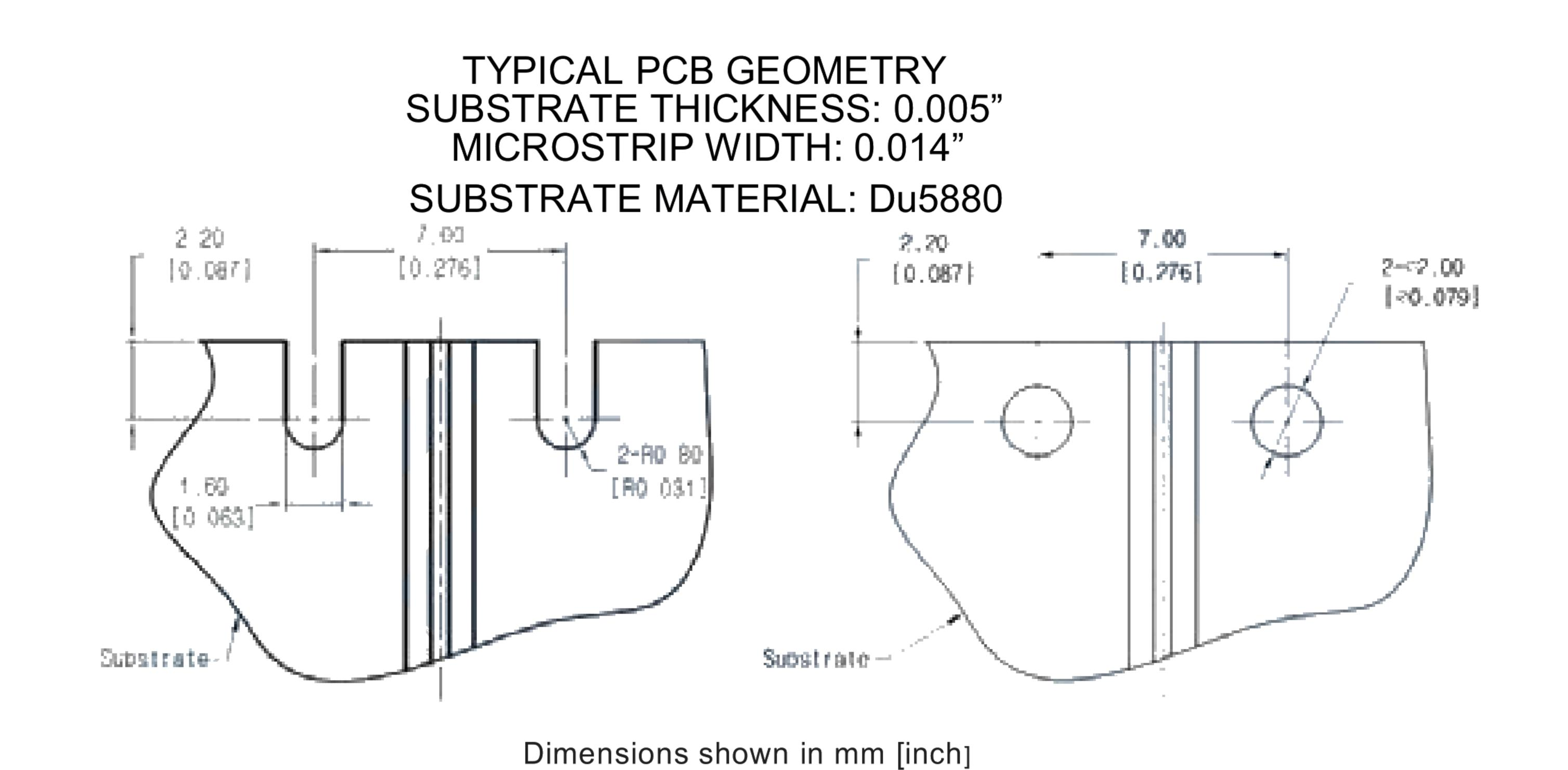
Click the following link (or enter part number in "SEARCH" on website) to obtain additional part information including price, inventory and certifications: SMA Female Connector Clamp/Solder (Captive Contact) Attachment End Launch PCB, Microstrip/Coplanar Launch, 0.005 inch ET11366
