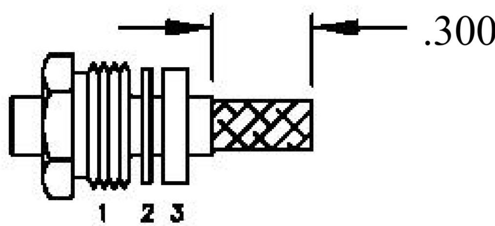
2. FORM BRAID OVER CLAMP NUT (4). TRIM BRAID BACK TO SHOULDER. CUT DIELECTRIC & CENTER CONDUCTOR TO DIMENSION SHOWN. DO NOT NICK CENTER CONDUCTOR. SOLDER CONTACT TO CENTER CONDUCTOR. REMOVE EXCESS SOLDER. DO NOT OVER HEAT DIELECTRIC. INSERT CABLE ASSEMBLY INTO BODY & TIGHTEN.
