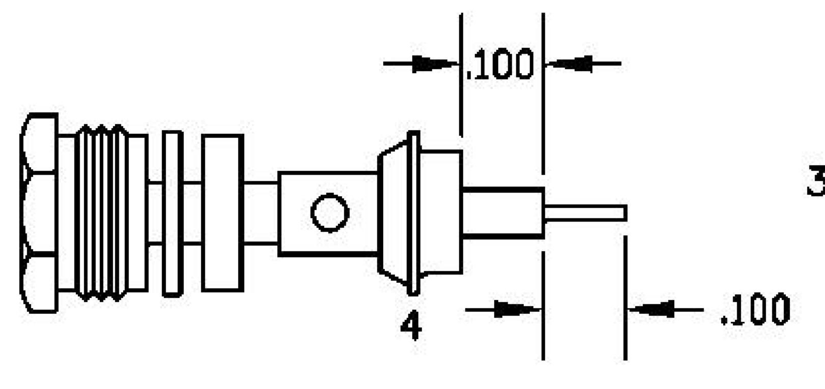
STRIP CABLE AS SHOWN IN ASSEMBLY (B). SOLDER CONTACT TO CENTER CONDUCTOR. SLIDE ASSEMBLY FORWARD & TIGHTEN TO
