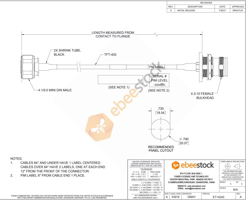
4.1/9.5 Mini DIN Male to 4.3-10 Female Bulkhead Low PIM Cable 60 Inch Length Using TFT-402 Coax Using Times Microwave Components
