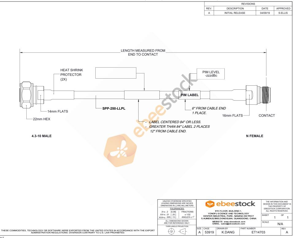
Plenum 4.3-10 Male to N Female Low PIM Cable 150 cm Length Using SPP-250-LLPL Coax Using Times Microwave Parts
