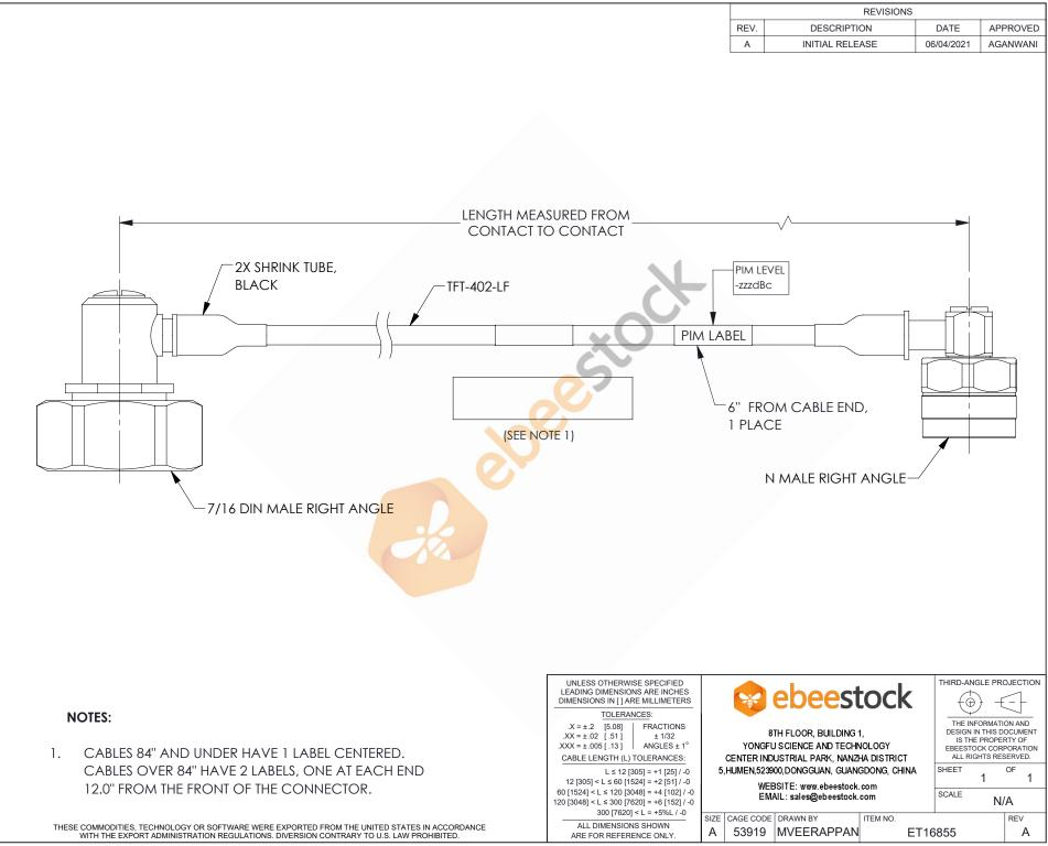
7/16 DIN Male Right Angle to N Male Right Angle Low PIM Cable 50 CM Length Using TFT-402-LF Coax Using Times Microwave Components
