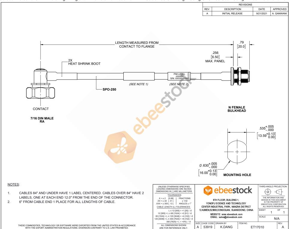
Outdoor Rated 7/16 DIN Male Right Angle to N Female Bulkhead Low PIM Cable 150 CM Length Using SPO-250 Coax Using Times Microwave Parts
