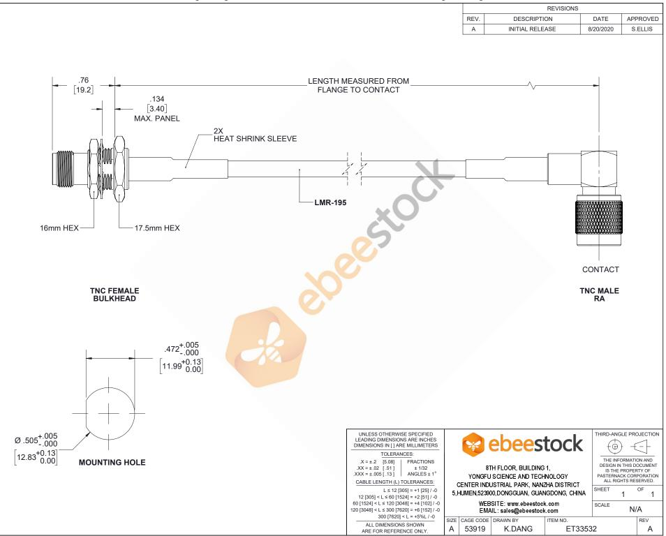
TNC Male Right Angle to TNC Female Bulkhead Cable 150 cm Length Using LMR-195 Coax
